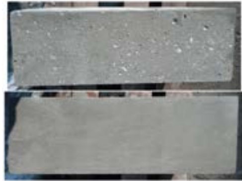
Figure 2: Concrete sample before and after sacking.
